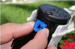
1. Insert the plastic end of the Hunter adjustment wrench into the lifting socket of the rotor and turn 90 degrees. Pulling up the riser will allow access to the nozzle port for
