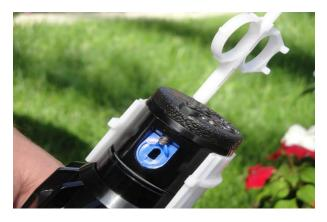
3. The triangle on the rubber cover will always indicate the location of the nozzle and direction of the water's flow, when the rotor is retracted. After the nozzle is installed, turn the adjustment screw a quarter turn clockwise to hold the nozzle into place. Anymore than a quarter rotation of the radius reduction screw will result in a minimized radius.
