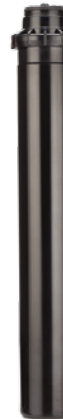
PGP-12 Overall height: 43 cm Pop-up height: 30 cm Exposed diameter: 4.5 cm Inlet size: ¾"
